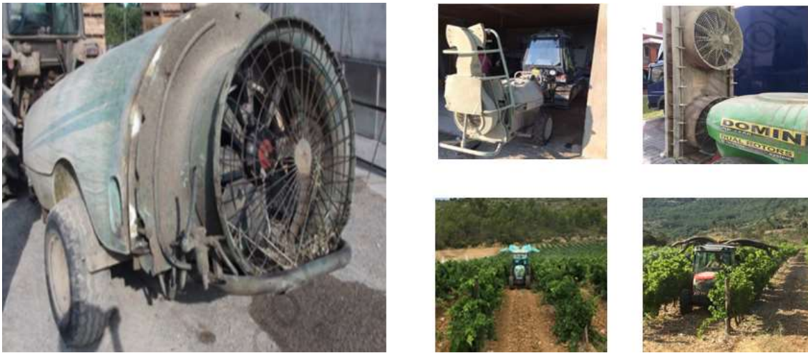
Figure 4: Sprayer classification; image on the left is 'Balleste' radial sprayer whilst those on the right are examples of sideways sprayers (e.g. 'Dragone', 'Dominiak', 'Pulveman' and 'Calvet Pneumatic')
