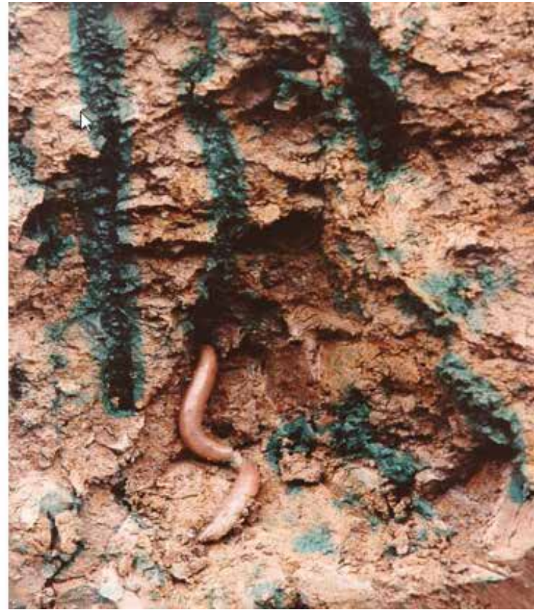
Figure 7: Water flow pattern in a soil profile (left side) and staining pattern of macropores (right side) made visible via infiltration experiments with colour tracer (Ref. 9)
