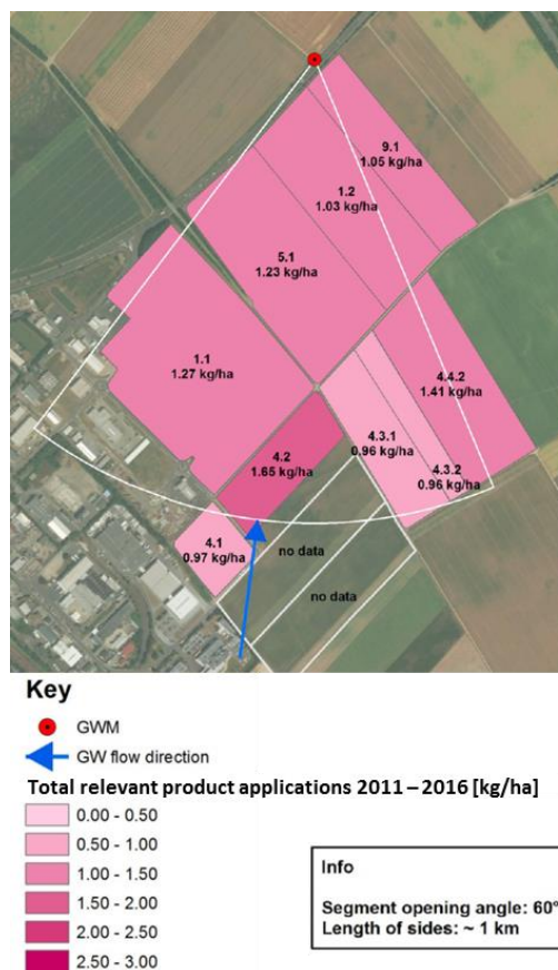
Figure A2-3. Well location, fields in well vicinity and product use history (ca. 20 associated products surveyed) up-hydraulic gradient of the monitoring well.
