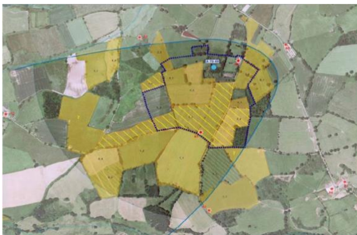
Figure 3-3. Example of the investigation of the recharge/catchment area of a well to collect the use history of an active substance, agronomic practices, soil information, and aquifer characteristics. The fields in yellow indicate cultivation of the targeted crop, yellow and thin hatching indicate cultivation of targeted crop and use of targeted compound the previous year, yellow and thick hatching indicate cultivation of targeted crop and use of targeted compound in this calendar year. The blue arc is the estimated recharge zone for the well (blue dot) and the black dotted line is the nitrate protection zone.
