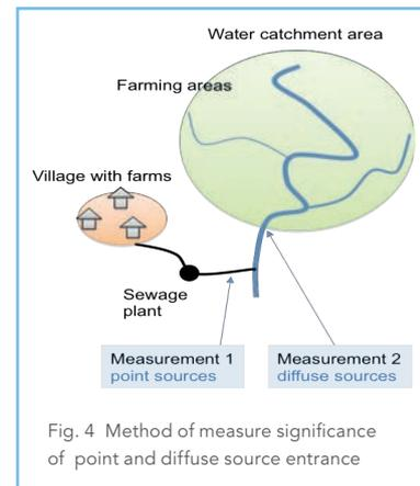
Fig. 4 Method of measure significance of point and diffuse source entrance
