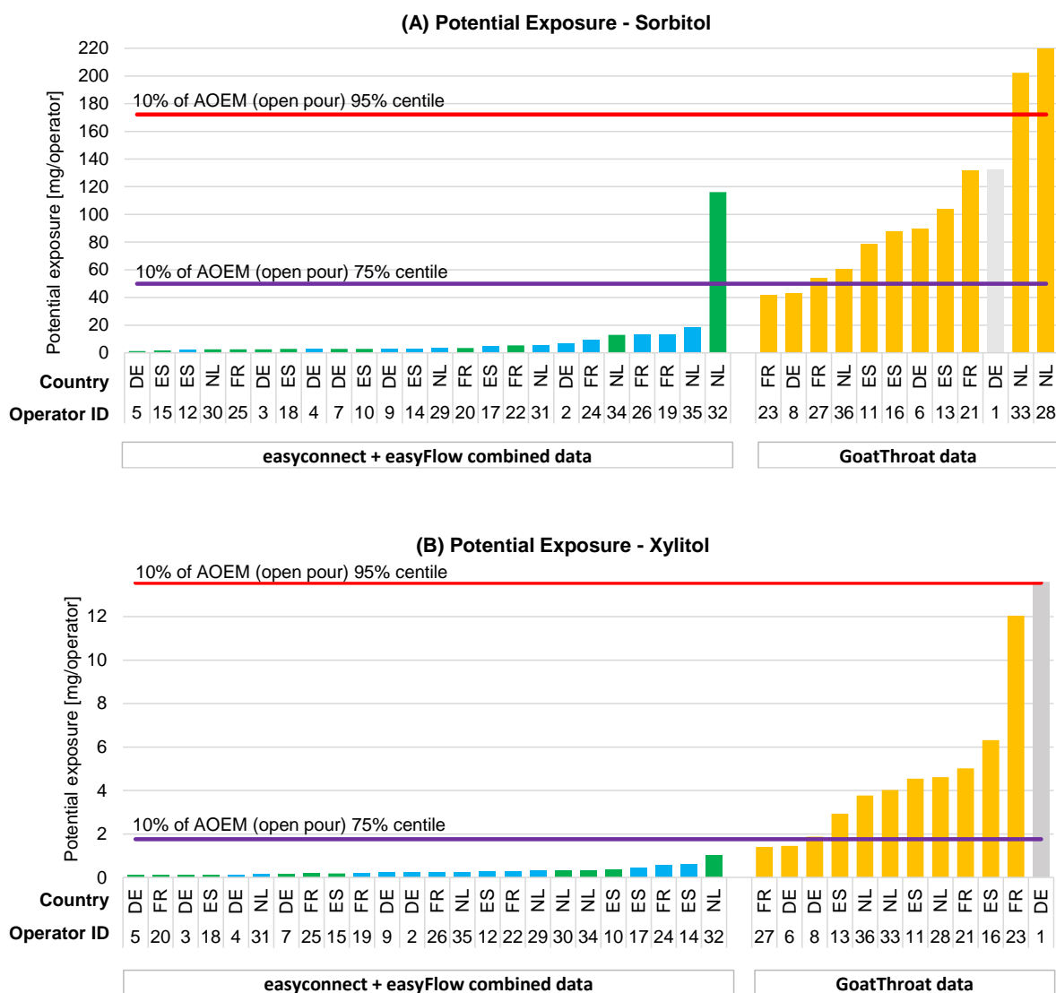
Fig. 3 Individual operator values for the potential exposure to (A) Sorbitol and (B) Xylitol. Green bars denote easyconnect, blue bars denote easyFlow and orange bars denote GoatThroat. The red line denotes 10% of the open-pour AOEM 95th centile and the purple line denotes 10% of the open-pour AOEM 75th centile.
