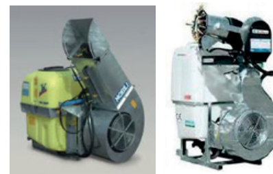
Fig. 13: Cannon sprayer, very vulnerable to drift.
