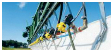
Fig. 14: Crop tilter opens crop for better spray penetration.
