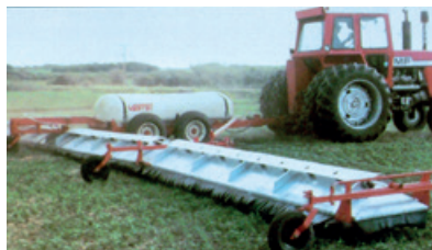
Fig. 23: Various shielded sprayers.
