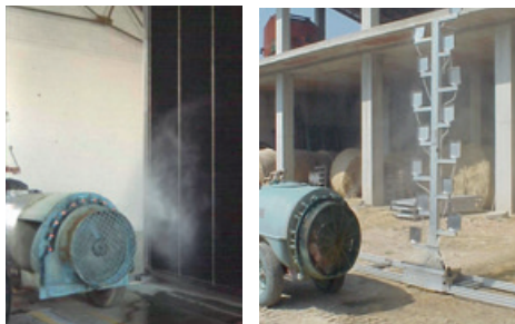
Fig. 28: Equipment to measure the vertical spray distribution.
