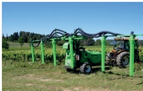
Fig. 19: Multi-row sprayer, a) with nozzles;
