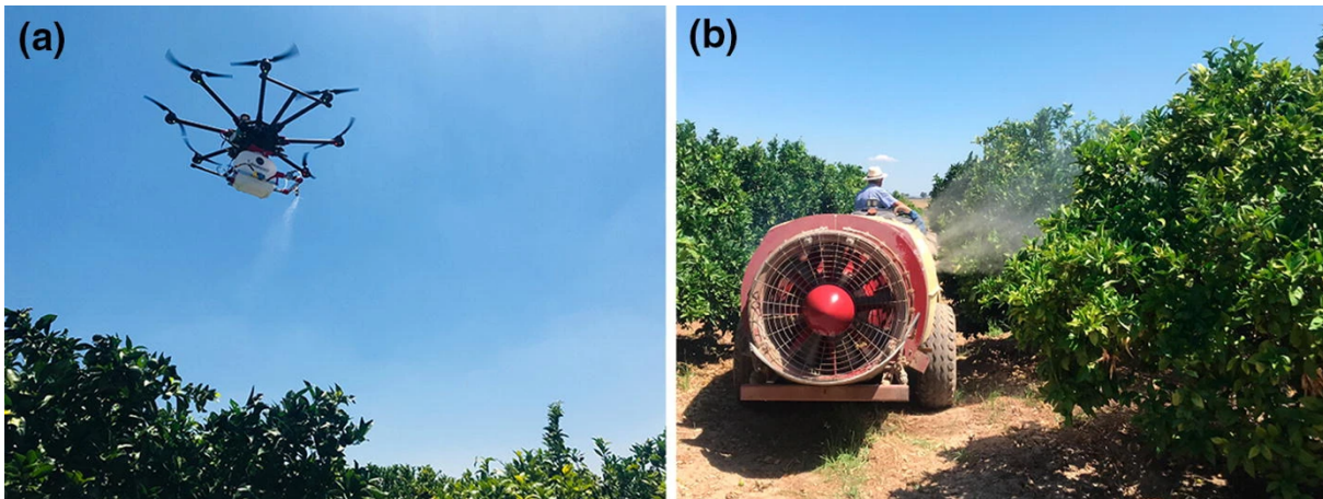
Figure 12: A UAV aerial application using a single-nozzle configuration. b Conventional spraying application of commercial product in orange trees using tractor+implement equipment. (From Jorge Martinez-Guanter et al., 2020: Doi:10.1007/s11119-019-09665-7)
